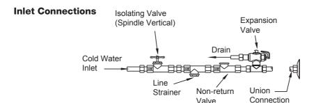
**Note:** a combined isolating valve/non-return valve/line strainer may be used. Expansion valve only required where local regulations demand.
